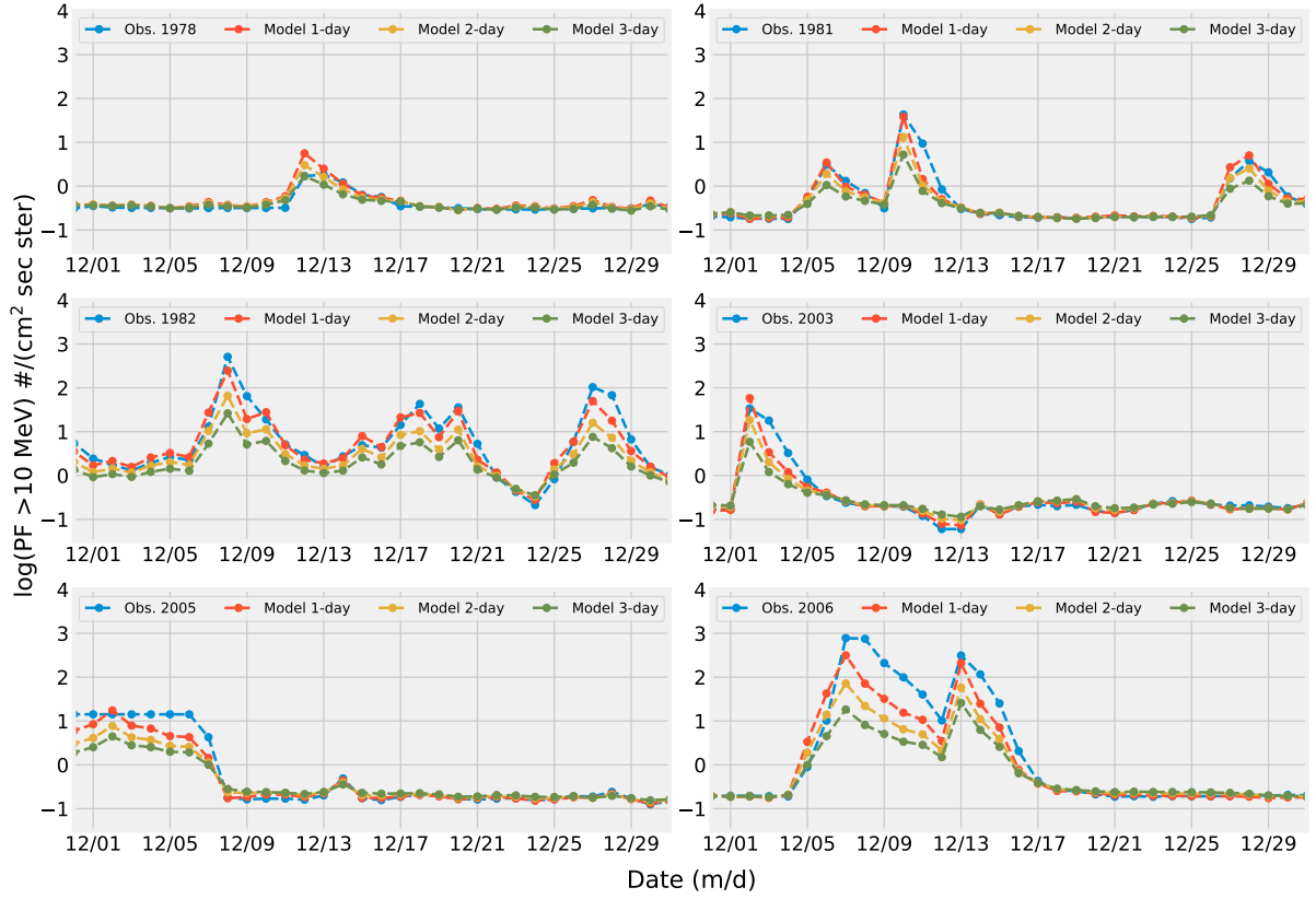
Figure 4.10: The model’s forecasts for the out-of-sample testing set for the >10 MeV channel are shown at forecast horizons of 1 day, 2 days, and 3 days ahead, using samples of data from December in selected years mentioned in the top-left side of the plots.
