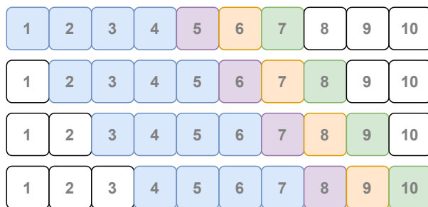
Figure 4.4: Illustration of the sliding window technique for a sample of 10 timesteps, where each number denotes a distinct time step. As an example here, the input horizon (blue color) length is 4 timesteps and the output horizon length is 3 timesteps. The input window slides 1 time step at a time across the entire data sequence to generate 4 distinct input and forecast horizon pairs. The purple, orange, and green colors of the output horizon represent 1-day, 2-day, and 3-day ahead forecasting, respectively. The timesteps of 1-day ahead forecasting across the data sequences are then concatenated into a single timeseries list that is called 1-day ahead prediction. The same for 2-day and 3-day ahead.
